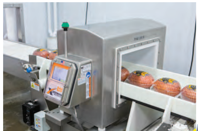
An Xtreme® metal detector safeguards cooked hams in the packaging process.
