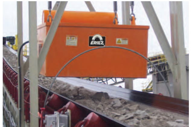
This suspended magnetic separator removes large unwanted metals from a conveyor moving aggregates.
