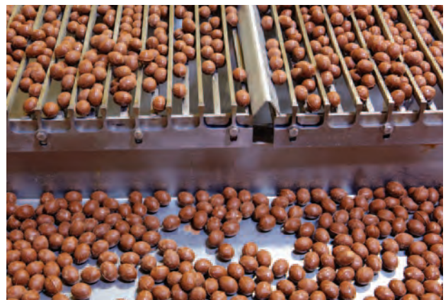
A vibratory feeder meters chocolate candies for final packaging.
